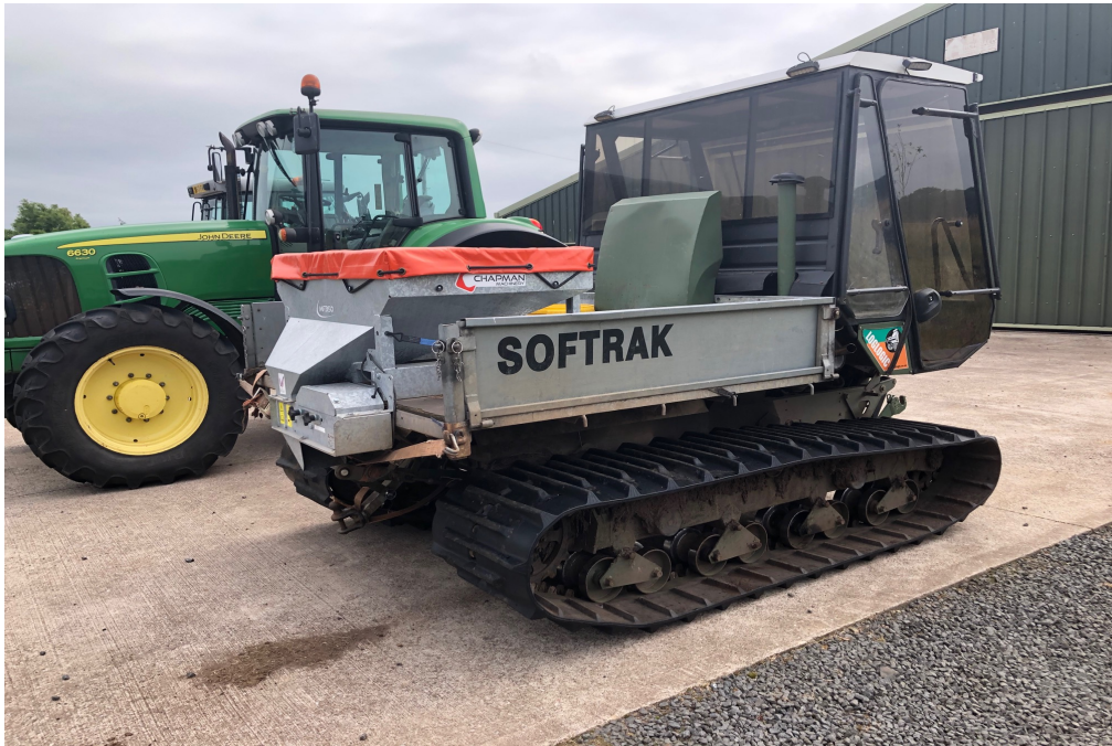
Low impact Softrak with mounted cob feeder
